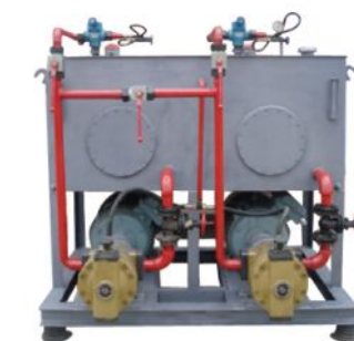
Hydraulic Pump Station 液压泵站
